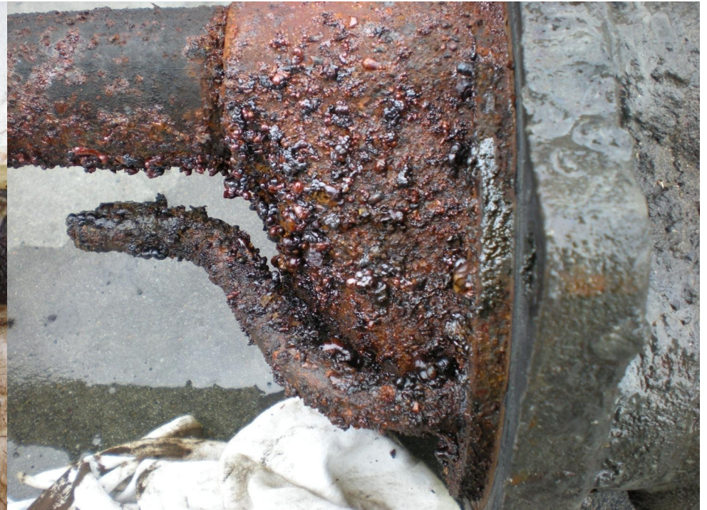
Submersible Pump Head (in vapor space -- never contacts fuel)
