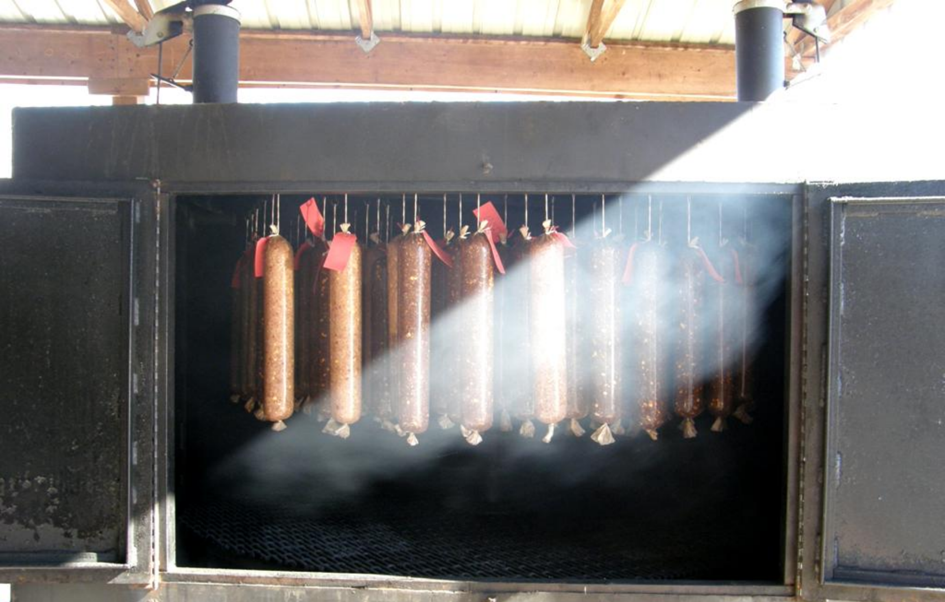
2,000 GALLON WATER TANK CONVERTED TO SMOKER
