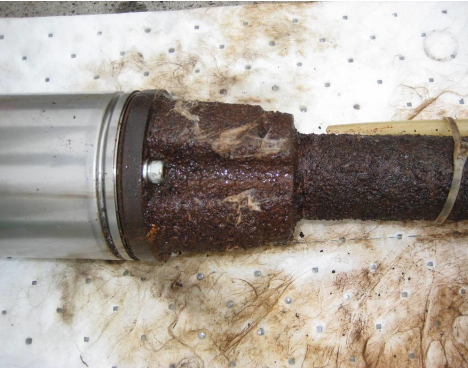
Submersible Pump & Riser (Left hand side is aluminum; Right hand side is steel)
