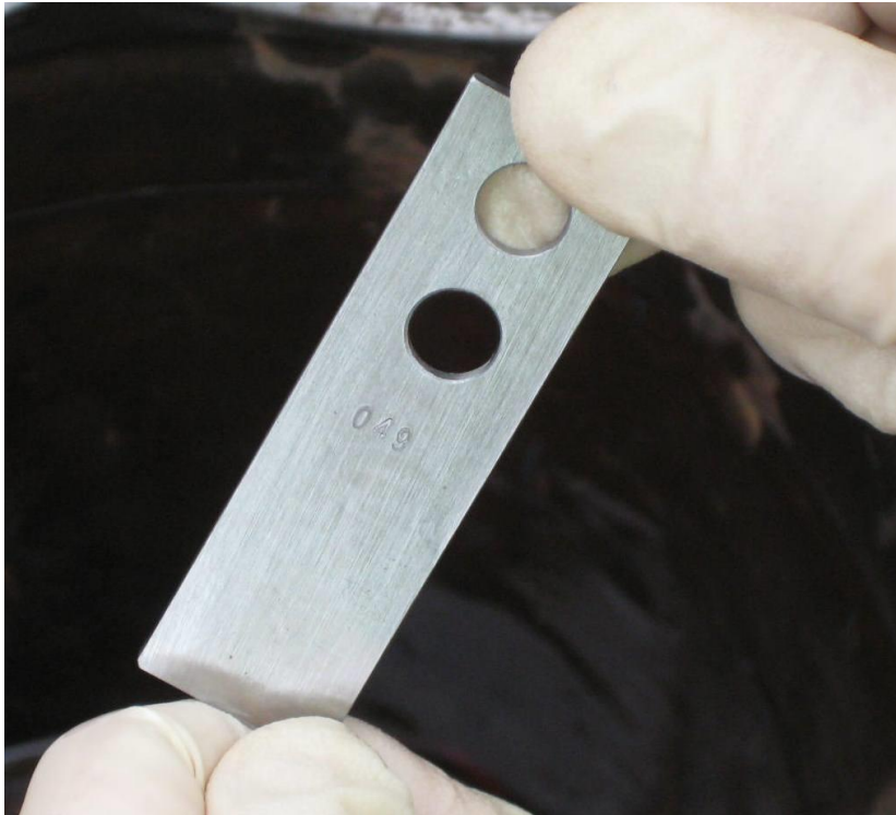
New steel corrosion coupon
