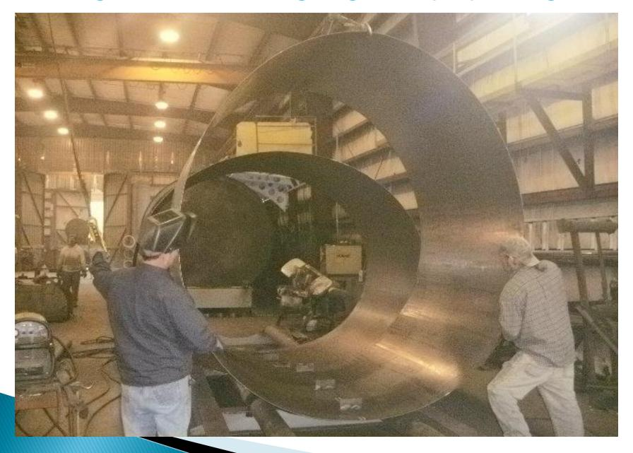
Weld the inside of the primary tank - Butt welding
